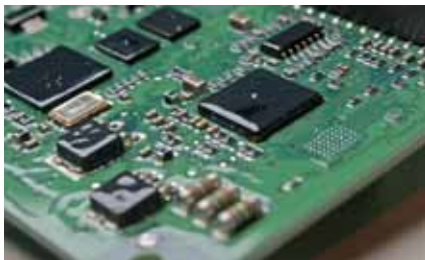
Coated control boards are available for harsh environments.
